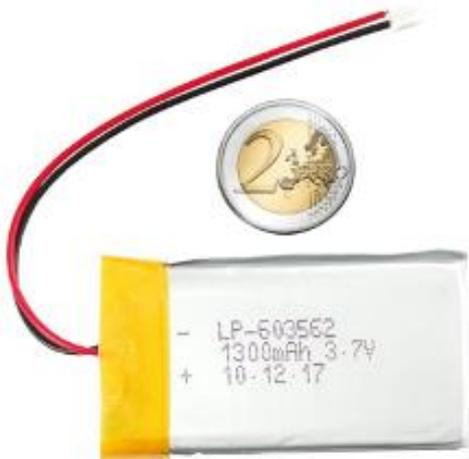
3.7V 1300mAh battery to power the Raspberry Pico inside your CanSat, without the USB cable.
