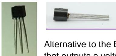
Alternative to the BMP280, the TMP36 is a basic analogue temperature sensor that outputs a voltage based on the ambient temperature around the sensor.
