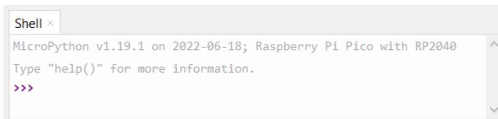
Thonny is now able to communicate with your Pico using the REPL (read–eval–print loop), which allows you to type Python code into the Shell and directly see the result.
