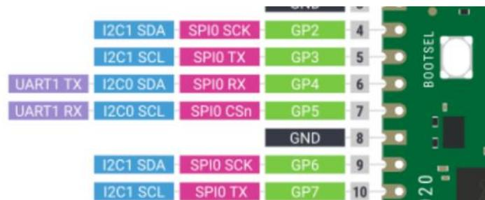
The Raspberry Pi Pico has two SPI interfaces and, as with the UART and I2C interfaces, it can be setup to use a variety of pins for the interface. For this lab we will use the GP2 to GP7 pins for the radio.
