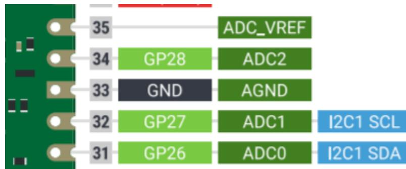
In their default configuration, the Pi ADCs will sample the voltage on the ADC input pin, this must be within the range of 0V to 3.3V. Once sampled, it converts the voltage to a number between 0 and 65,535 with a value of 0 representing 0V and a value of 65,535 representing 3.3V.
